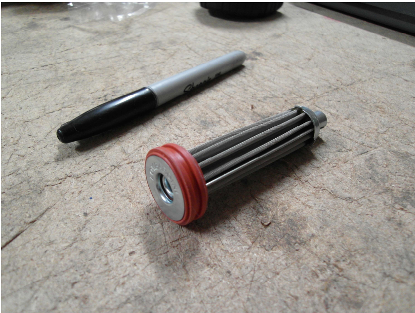
Diesel engine oil filter. Part number: 2175.155. Remember, it is cleanable/ reusable.
