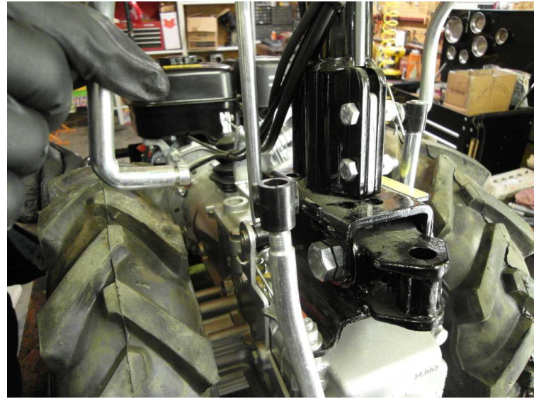
1) Remove pin & washer, Slide PTO control rod sideways out of plastic joint. Then, lift plastic joint off lower shift lever.
