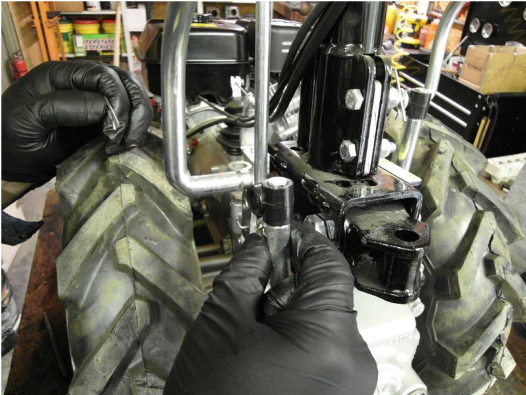
14) Reconnect outer shift levers at joint, sliding joint down onto the lower lever first, then the control rod into the joint. Re-install washer and then R-pin to secure.
