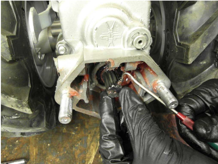
8) Remove old spring from hole in side of shaft with pick, little screwdriver, piece of wire, etc.
