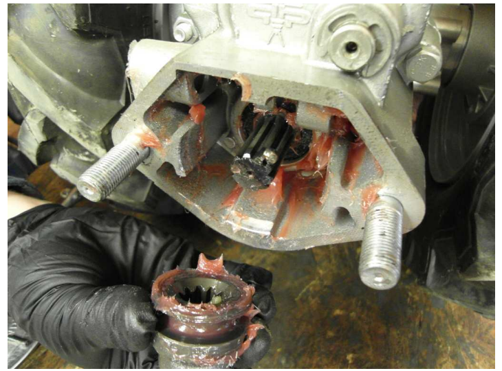
7) PTO coupler separated from PTO shaft. Note we placed detent ball in position on side of shaft for this picture. (this is a good time to remove the roll pins from the recess up in corner)
