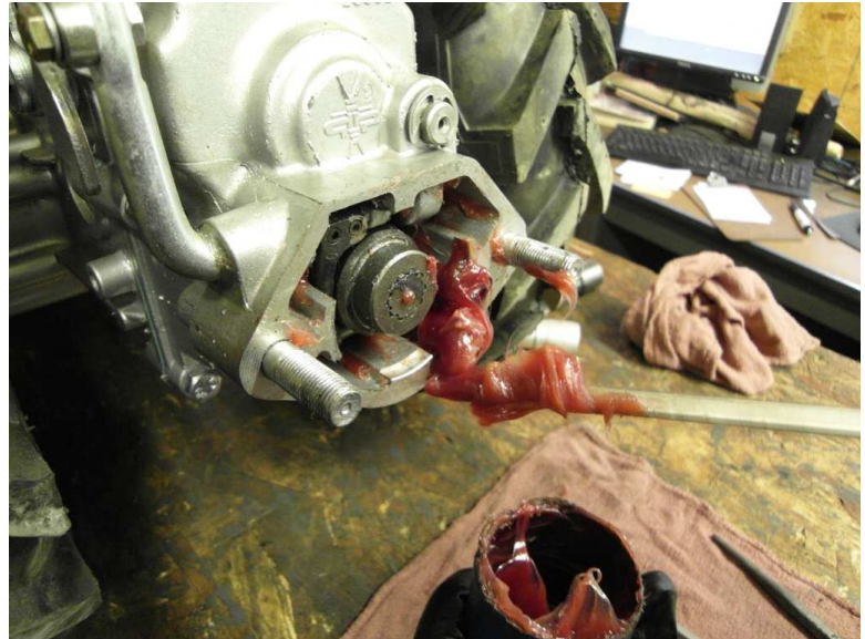
15) Re-pack PTO flange with general-purpose lubricating grease. (this can be done with a grease gun)
