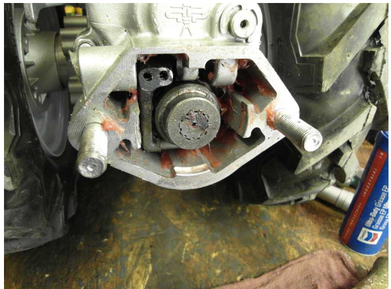
11) Reinstall inner PTO shift lever into PTO flange, aligning bottom "bar" of the lever inside the slot on the coupler.
