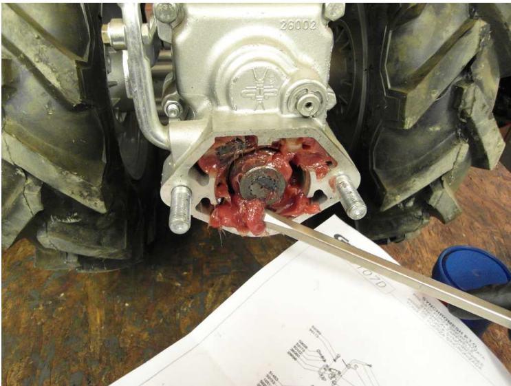
2) With implement / female Quick coupling removed from tractor, clean some grease out of PTO area so you can see inside.
