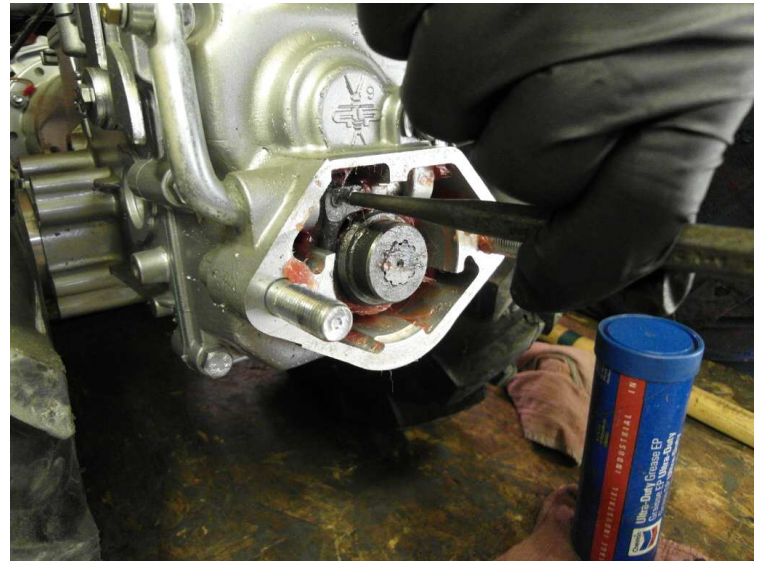
3) Drive roll pins through shift lever with 3/16" straight punch. The pins will fall through the other side into a recess in the housing, and can be easily retrieved after linkage is removed.
