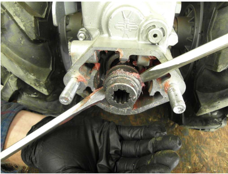
6) Pop PTO coupler off shaft with a couple of screwdrivers. Watch out for the detent ball & spring...the ball will pop out of the shaft when the coupler is removed.
