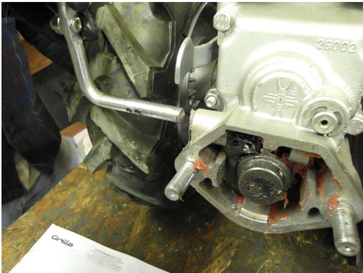
4) Slide outer PTO lever out of housing.
