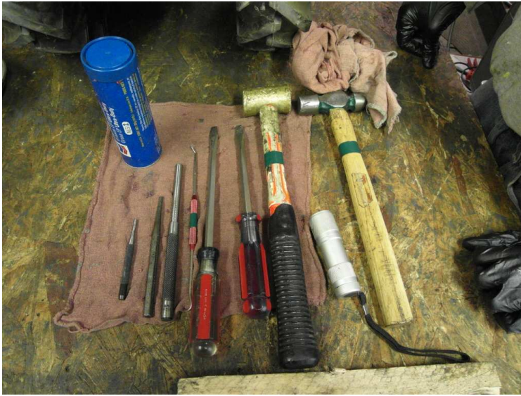
Tools needed for job (3/16" pin punch, screwdrivers, hammer [brass or steel], pick, grease) (you don't need the flashlight...)
