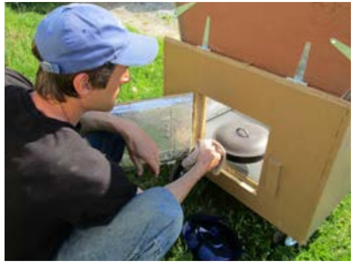
Joel and his daughter Sophie are shown with one of their solar ovens. This model includes a rear door for fast food removal and wheels for mobility.
