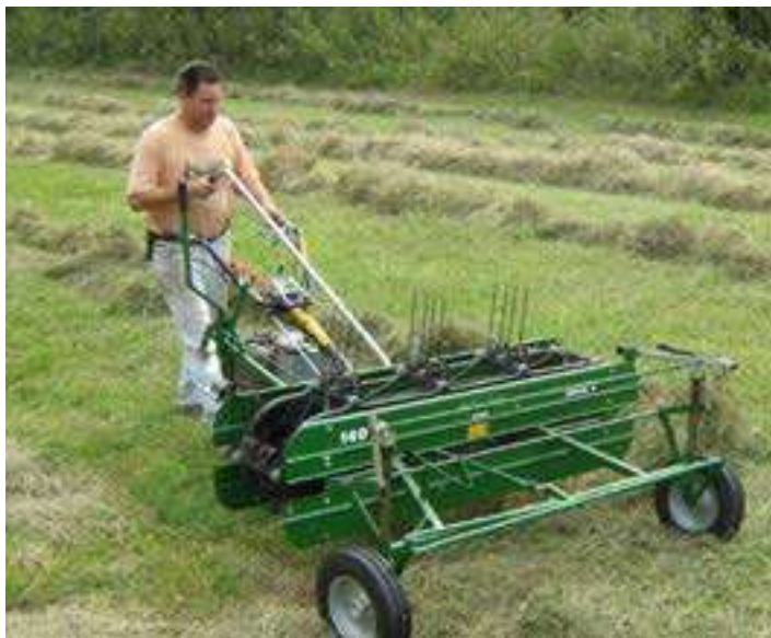
A walk-behind hay rake implement (left) gathers hay in 30 minutes per acre. A hay-baler implement (right) can make a bale per minute.
