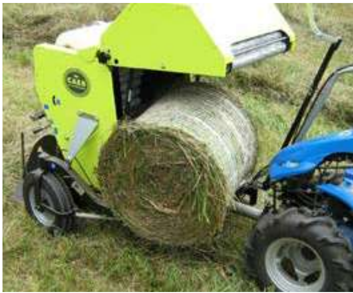
A walk-behind tractor hay-baler implement (left) produces 40- to 60-pound round bales, and you can stack up a trailer-load (right) in an afternoon.
