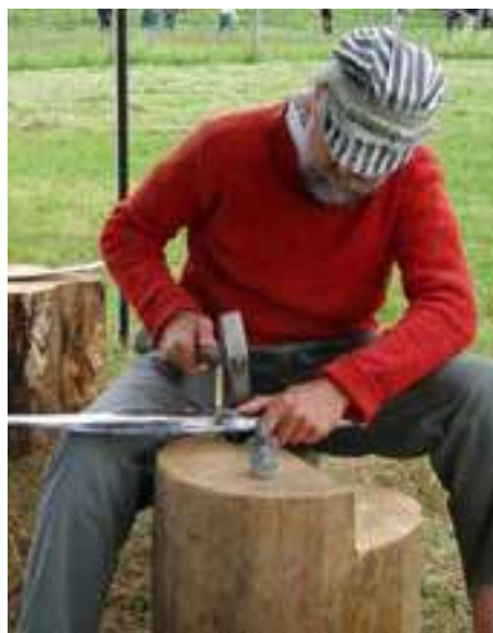
Occasionally peening your scythe with a special peening hammer will extend the life of your blade.
