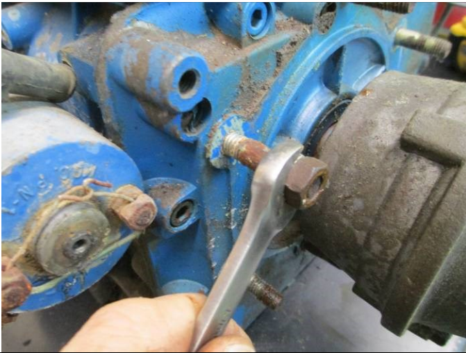
#7. USING THE “INNER” NUT, BACK THE STUD OUT OF THE ENGINE.
