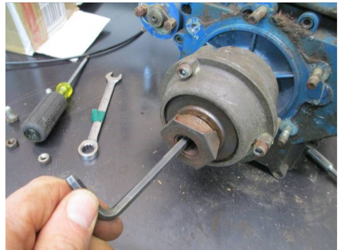
#10. INSERT A 6MM ALLEN WRENCH INTO THE HOLE IN THE CLUTCH; FEEL AROUND FOR THE BOLT-HEAD. (NOTE: On SEP/Mainline units, remove center bearing assy. from clutch [just slides out] and use a 13mm socket to remove center bolt)
