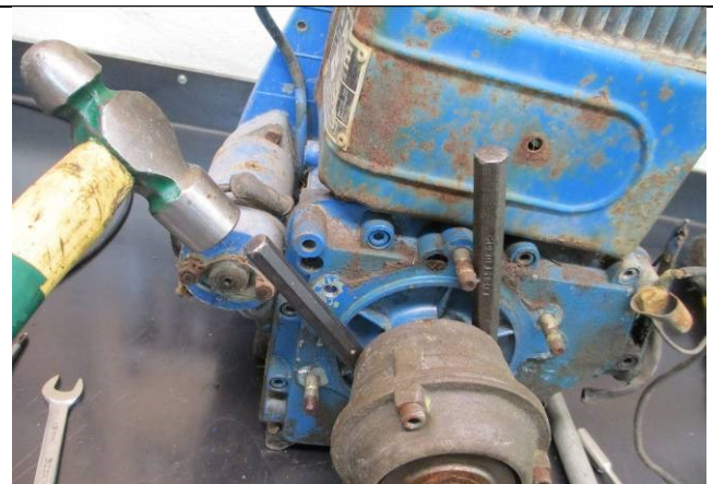
#12. NOW THAT THE BOLT IS LOOSE, THE CLUTCH MUST BE BROKEN FREE FROM THE TAPER-LOCK ON THE CRANKSHAFT. THIS CAN BE DONE BY WEDGING TWO LARGE COLD-CHISELS (METAL-CUTTING CHISELS) BETWEEN THE CLUTCH HOUSING AND THE ENGINE CRANK-CASE — ONE ON EITHER SIDE OF THE CRANKSHAFT— AND HITTING ONE...
