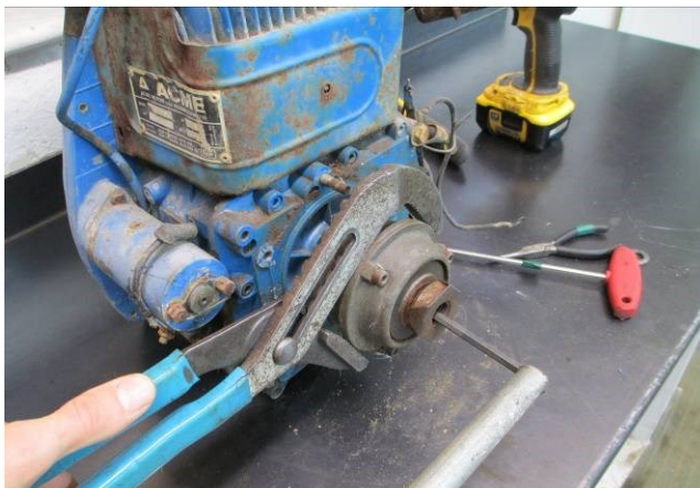
#11. USING A LARGE CHANNEL-LOCK PLIERS, STRAP-WRENCH, PIPE-WRENCH, ETC. HOLD THE OUTER HOUSING OF THE CLUTCH TO KEEP IT FROM TURNING WHILE LOOSENING THE BOLT INSIDE THE CLUTCH. NOTE: I HAVE A PIPE ON THE “SHORT” END OF THE ALLEN WRENCH FOR EXTRA LEVERAGE. BOLT IS STANDARD THREAD, NOT LH.
