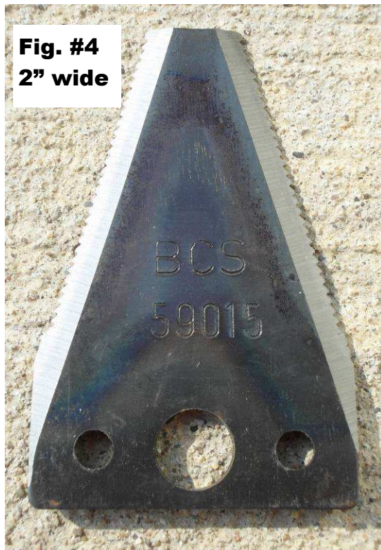
Figure 4A: “Bolt-on” type blade; note that there is no “serrated plate” on the blade to attach the blade coupling to...instead, the bolt-holes are drilled directly in the “strip.”
