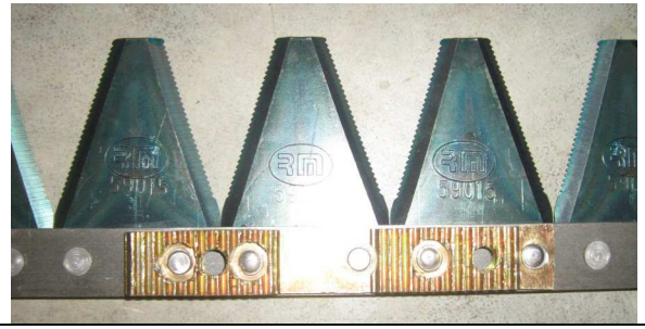
Figure 4B: “Standard” type blade; note the “serrated plate” riveted to the blade to attach the blade coupling onto, with threaded bolt-holes in plate for mounting blade coupling.
